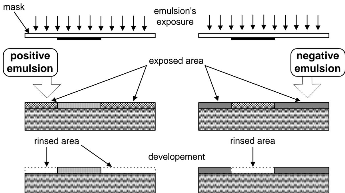
**Fig. 2. The difference between the results of exposure of positive and negative photoresist through the same mask.**
