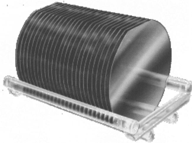
*Fig.2. The wafers in a quartz boat*
