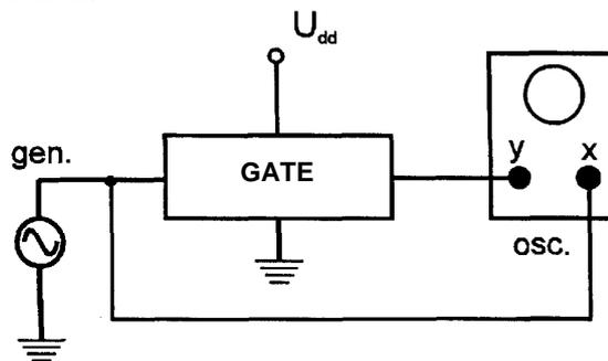
Fig. 5. Diagram of measurement circuit for transient characteristics (the oscilloscope method)
