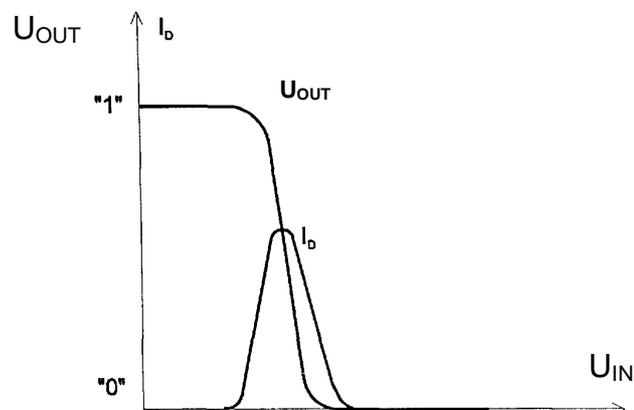
Fig. 2. Transient characteristics of the inverter
