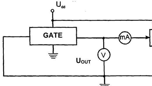
Fig. 8. Measurement circuit for output characteristic in the high state on the output
