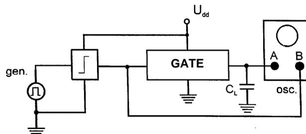
Fig. 9 Measurement circuit for propagation times
