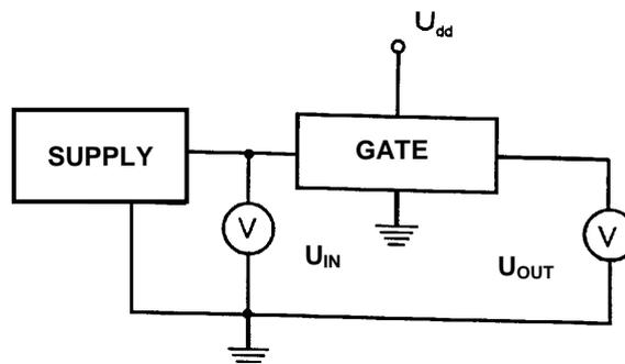
Fig. 6. Diagram of measurement circuit for transient characteristics ('point by point' method)
