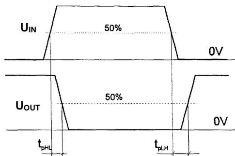
Fig.4. Time plot for the input and output voltages during switching
