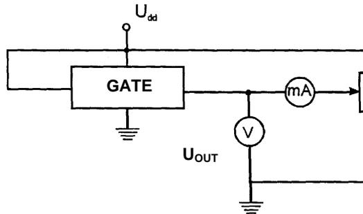
Fig. 7. Measurement circuit for output characteristic in the low state on the output
