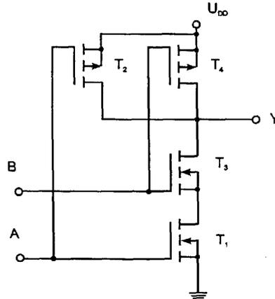
Fig.3. CMOS NAND gate with two inputs
