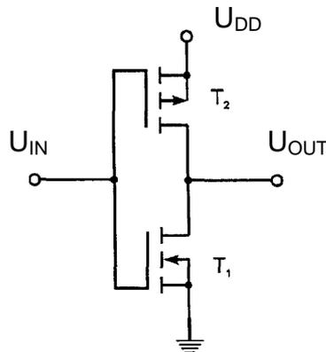
Fig. 1. The basic scheme of the inverter
