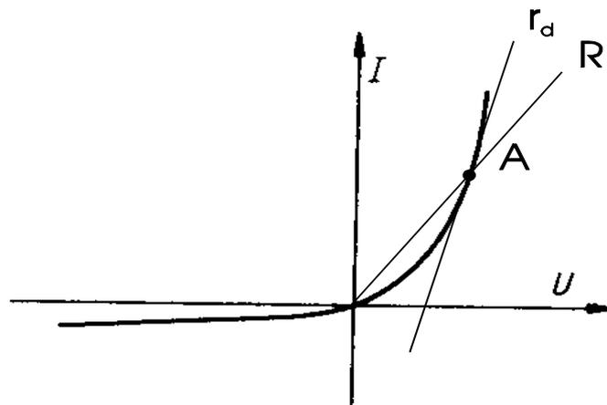
Fig.1. DC volt-ampere characteristic of the ideal diode.
