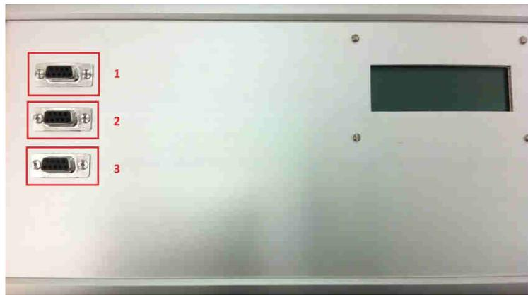
Fig.11. Front of the measurement panel with marked sockets no.1 – DC characteristics, no.2 – switching, no. 3 – Junction capacitance
