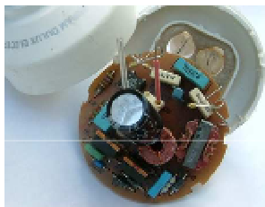
Photo 3. Electronic ignition system for compact fluorescent lamp
