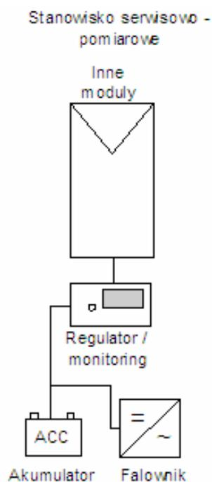
Fig 1 Scheme of small off-grid PV system, used in Photovoltaic Laboratory .
