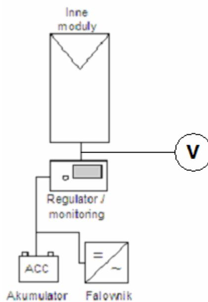
Fig 2 Measurements of PV module voltage/current
