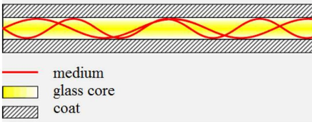
*Fig. 2. Graded index fiber*
