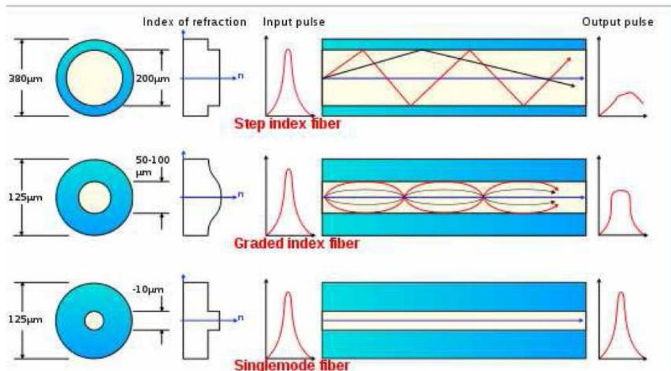
Fig. 4. Optical fiber types
