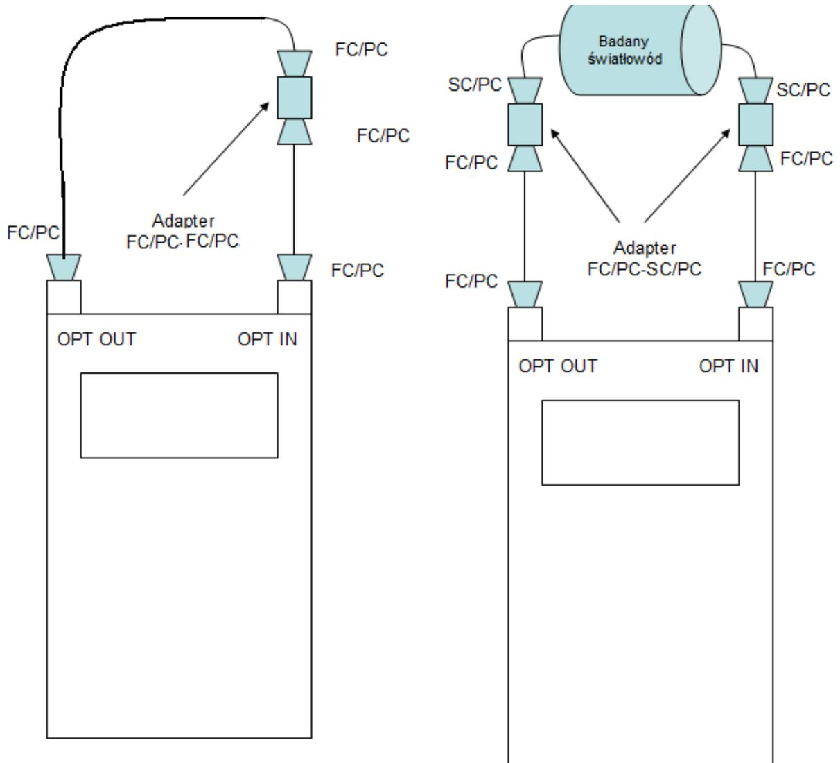
*Fig.5.a) meter calibration b) measurement of fiber attenuation*
