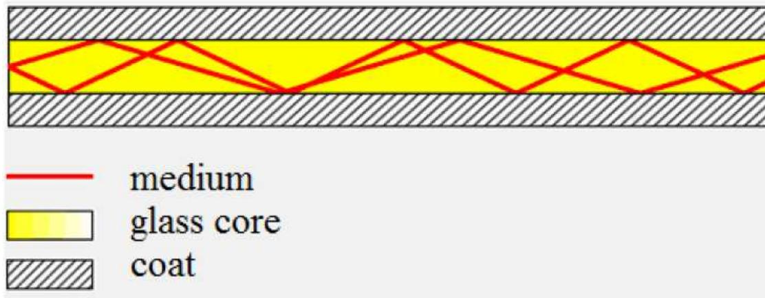
*Fig.3. Step index fiber*
