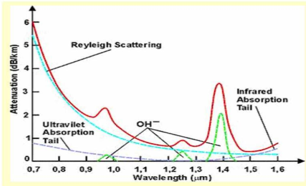
Fig 1. Quartz fiber attenuation dependence on the wavelength
