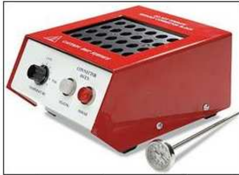
Fig.10 Oven used for heating the connectors ( http://theeraj1986.hpage.co.in/sc_pc_12756543.html )
